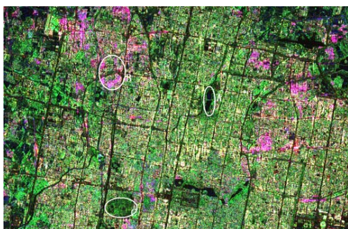
Fig.2 Pauli-basis image of the original fully polarimetric data over Beijing area
