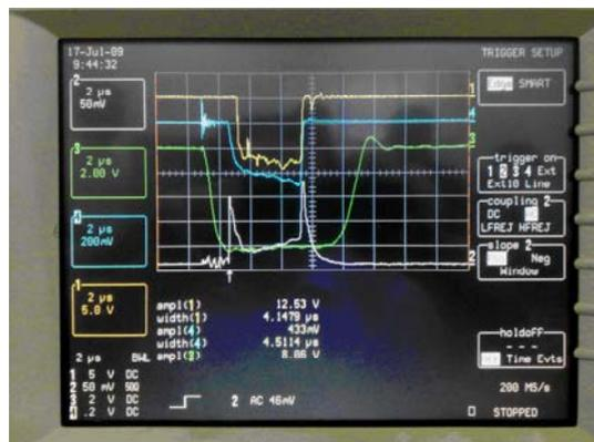
Fig.6 Tested waveform of thermionic cathode RF gun
