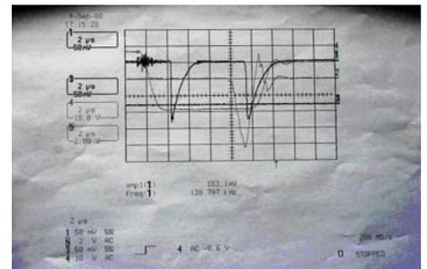
Fig.9 Spontaneous emission signal(channel 2)
