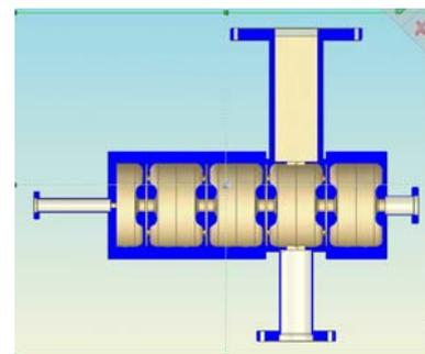
Fig.1 Schematic of the RF-gun
