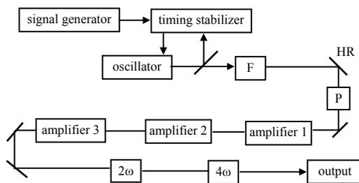
Fig.4 Cathode-driving laser system
