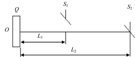
Fig.3 Schematic of the emittance measurement
