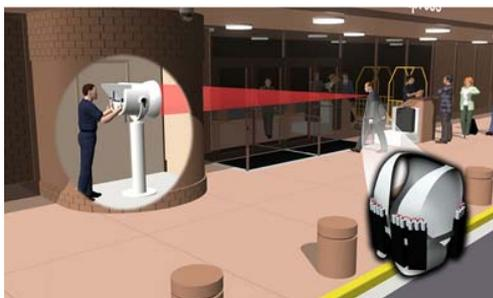
Fig.5 Conceptual drawing showing the operation of a sub-millimeter wave imaging system for the detection of concealed explosives or other weapons
