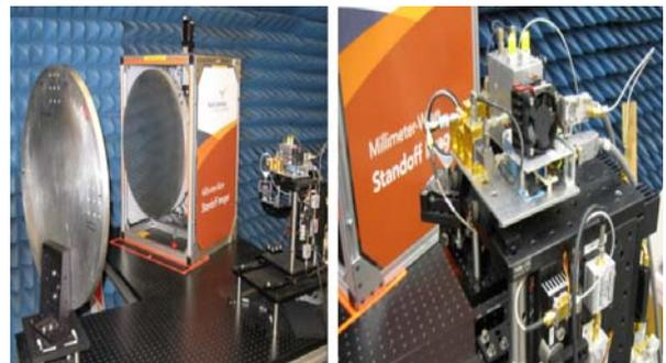
Fig.6 Photographs of the experimental prototype imaging system
