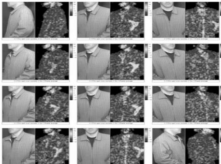
Fig.13 Sample images of a person with cable tie gun hidden under jacket, color scale is in dB
