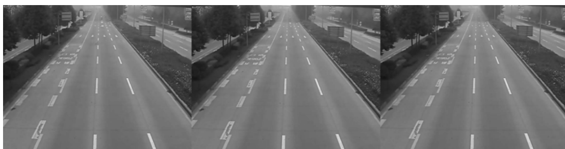
Fig.3 From left to right is a 10 frames learning, 10 frames learning plus 10 frames update and 20 frames learning background model of the same real-world road using proposed method in this thesis. 图 3 从左到右依次是本文方法的 10 帧模型, 10 帧模型更新 10 帧, 以及 20 帧模型的背景
