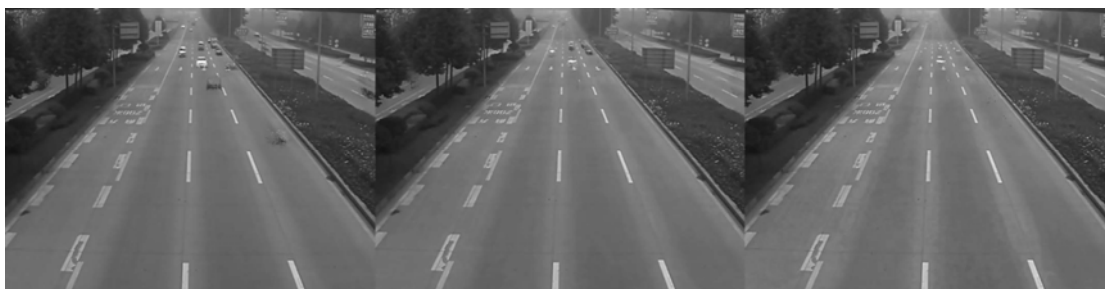
Fig.2 From left to right is a 20, 80 and 150 frames updated real-world road background model using an Gaussian mixture model 图 2 从左到右依次为混合高斯模型背景更新 20 帧, 80 帧与 150 帧后的背景模型
