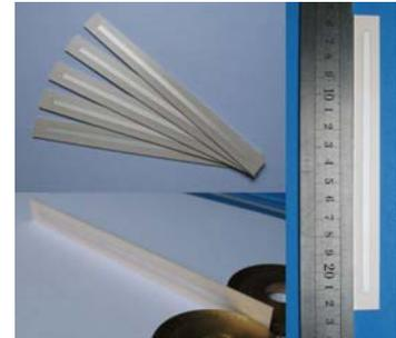
Fig.1 Solid-state ceramic planar transmission lines
