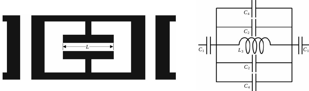
Fig.2 Structure parameters and the equivalent circuit model of CELC 图 2 CELC 单元参数及等效电路
