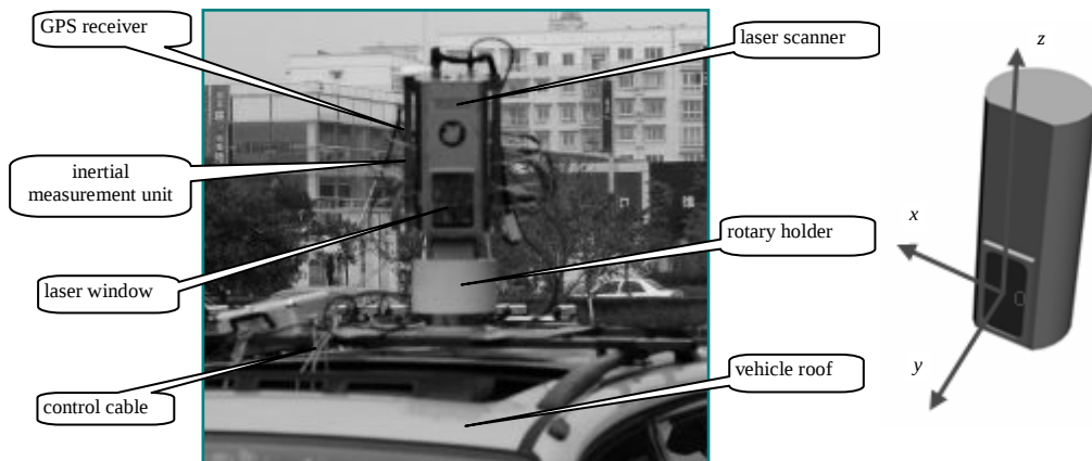
Fig.1 Vehicle-borne light detection and ranging system and local coordinate system of laser scanner
