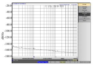
Fig.4 Phase noise test results of the 80 MHz crystal oscillator 图 480 MHz 晶振相噪测试结果
