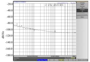
Fig.7 Phase noise test results of the frequency synthesizer with the traditional signal PLL
