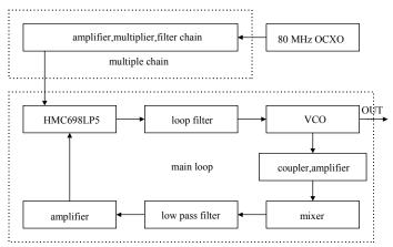
Fig.2 Diagram of the C-band frequency synthesizer with low phase noise 图 2 C 波段低相噪频率合成器原理框图
