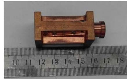
Fig.7 Experimental sample of tapered waveguide
