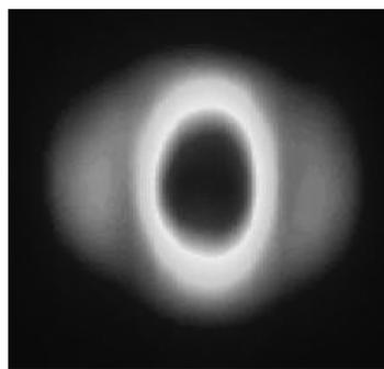
(b) output electric field distribution at  $L=20$  mmFig.8 Output electric field distribution of  $\phi 3.58-\phi 10$  tapered waveguide图8  $\phi 3.58\sim\phi 10$  过渡波导输出端电场分布
