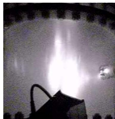
Fig.4 Image of discharge with microwave pulse width 1 \mu\text{s} under 300 Pa
