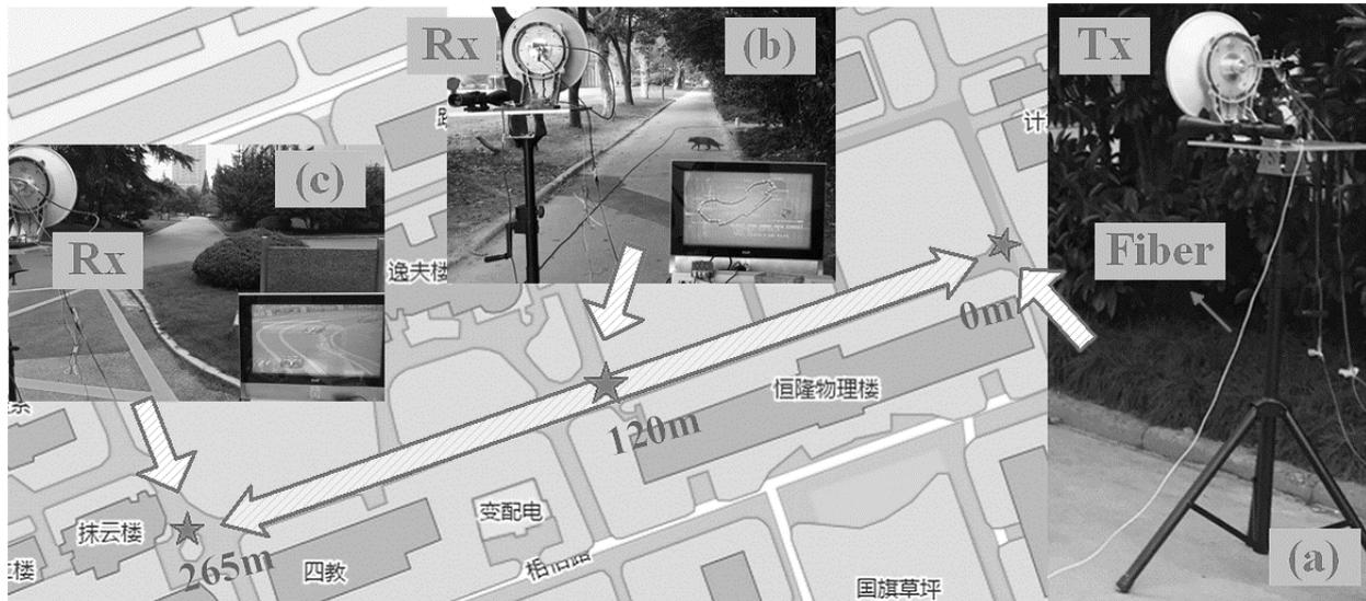
(a) transmitter at 0 m (b) receiver at 120 m (c) receiver at 265 m
