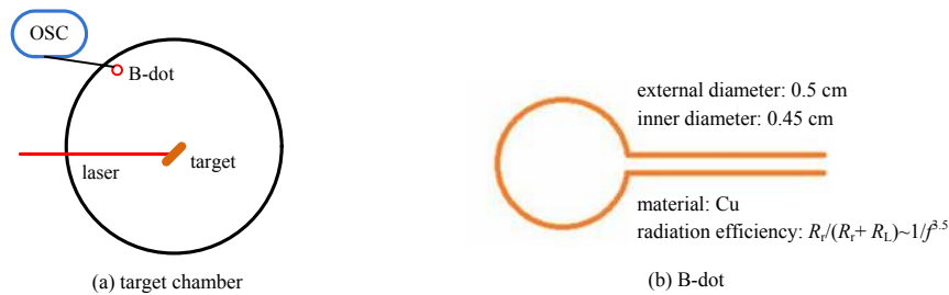
Fig.2 Illustration of measuring electromagnetic pulse in target chamber(a) and B-dot(b) 图 2 靶场内电磁波测量示意图(a),以及环形 B-dot 示意图(b)
