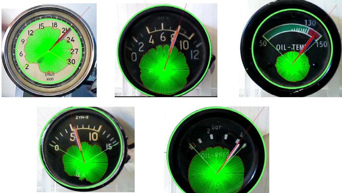
Fig.9 Pointer extraction results for different types of instrument
