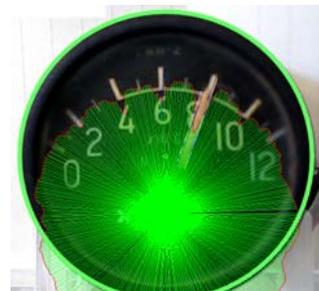
Fig.6 Pointers acquired by the method of the grey projection based on the polar center
