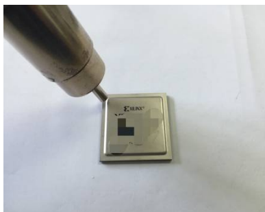
Fig.7 Heat gun with non-hermetic flip chip shell around the edges 图 7 热风枪喷吹非气密倒装芯片外壳四周边缘
