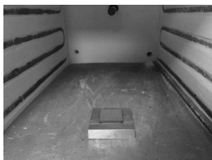
Fig.10 Flip chip removal of under-fill (epoxy resin) under high temperature 图 10 倒装芯片高温去除下填料(环氧树脂)
