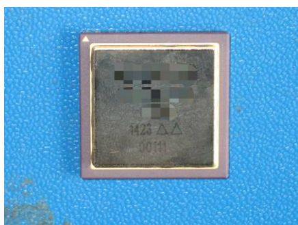
Fig.5 Hermetic encapsulation ceramic flip chip assembly integrated circuit 图 5 气密封装陶瓷倒装芯片组装集成电路
