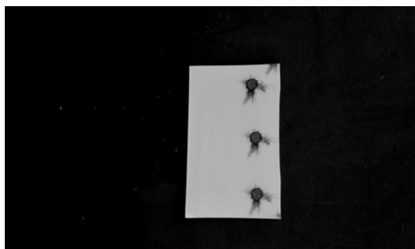
Fig.6 Display of the far-field laser spot 图6 激光远场光斑测试图
