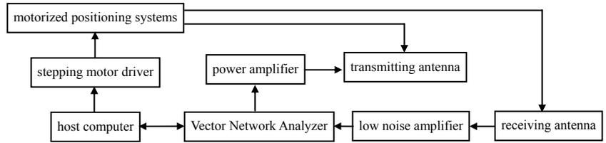
Fig.1 Configuration of the 0.14 THz imaging system
