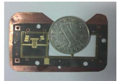
Fig.7 Picture of filter substrate
