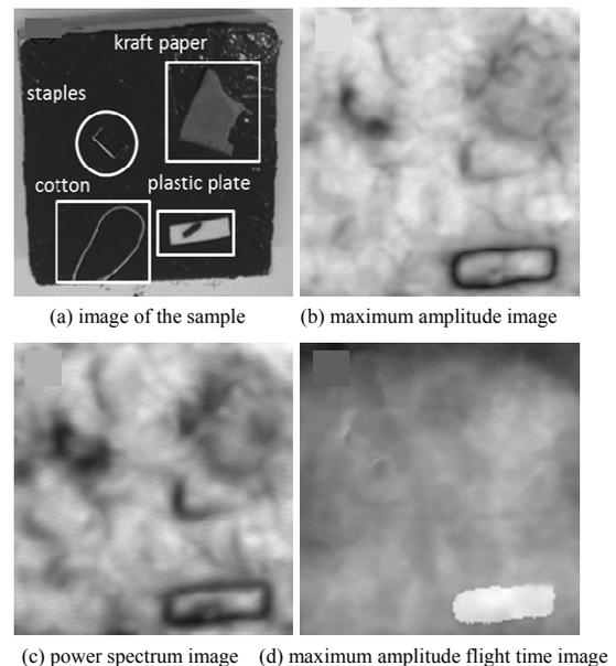
Fig.2 The views of the sample and reconstruction
