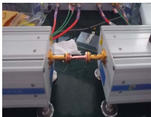
Fig.6 Photo of the wideband window test
