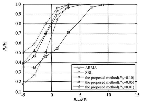
Fig.2 Probability of correct detection versus SNR
