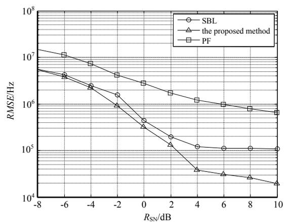
Fig.6 RMSE of frequency estimation versus SNR
