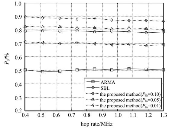
Fig.4 Probability of correct detection versus hop rate
