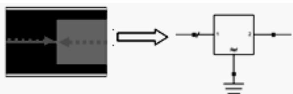
Fig.6 HFSS and ADS models for stepped impedance transformation structures with microstrip transmission lines
