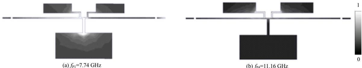
Fig.3 Normalized surface current distribution
