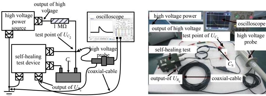
Fig.6 Self-healing test system based on the circuit in Fig.2
