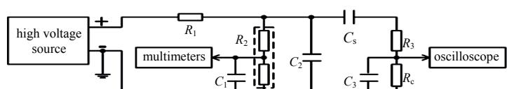
Fig.2 Principle of self-healing test circuit
