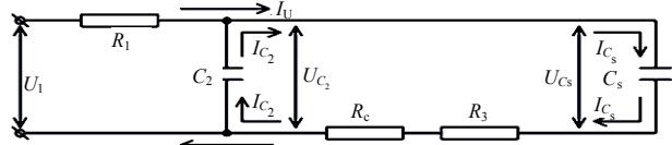
Fig.3 Voltage and current characters of the working self-healing test circuit
