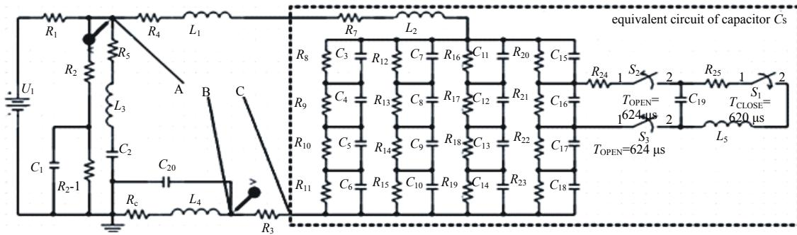
Fig.4 Simulation model of self-healing test circuit
