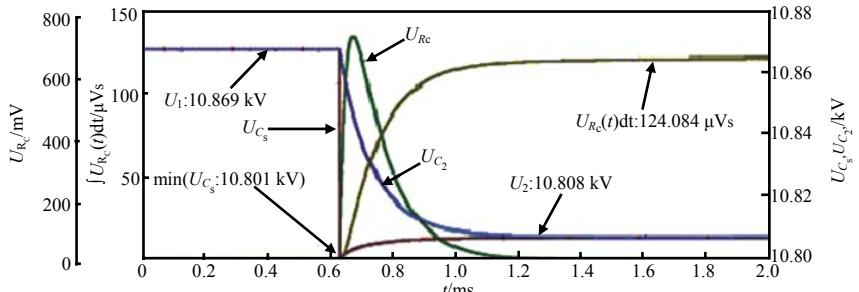
Fig.5 Simulation results of self-healing test circuit
