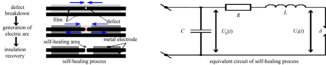
Fig.1 Self-healing process of metalized film capacitor and its equivalent circuit
