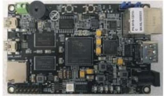
Fig.3 Fast dehazing processing board for video image based on SoPC
