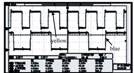
Fig.4 Test waveform of TTL serial port receiver
