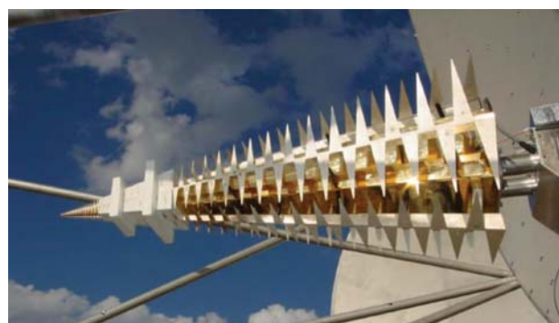
Fig.1 Log periodic antenna feed developed for ATA(0.5~11.2 GHz) 图 1 ATA 对数周期馈源(0.5~11.2 GHz) [21]
