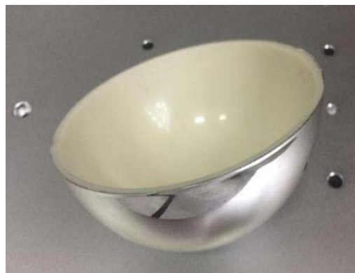
Fig.1 Aluminized ABS hemispherical shell 图 1 镀铝 ABS 半球壳
