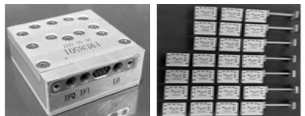
Fig.7 Photo of V-band miniaturized integrated receiving front-end
