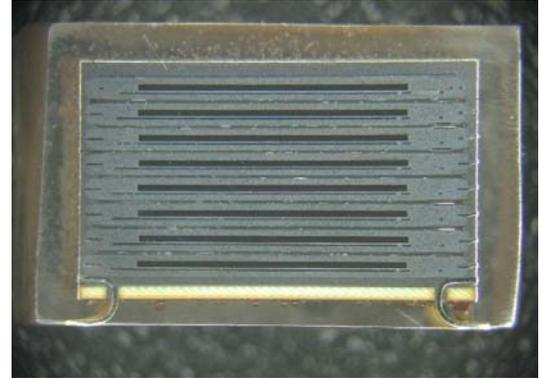
Fig.7 Typical cross-sectional structure of the test sample
