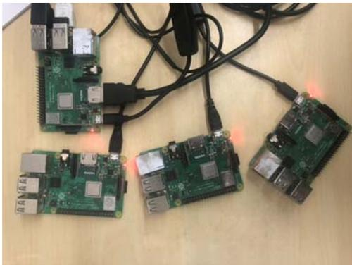
Fig.6 Raspberry Pi testbed
