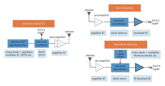
(a) Transceiver architecture of terahertz high speed wireless communication system based on all electronics
