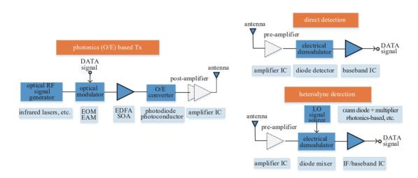
(b) Transceiver architecture of terahertz high speed wireless communication system based on photoelectric hybrid
