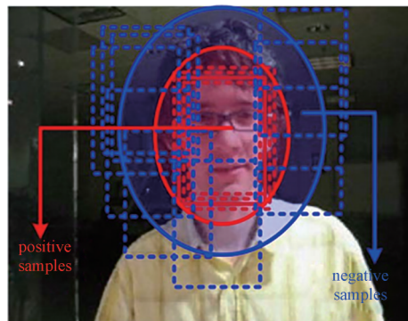
Fig.2 Schematic diagram of positive and negative sample collection
