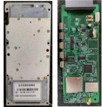
Fig.14 Prototype of ISAC module
