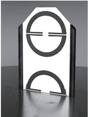
Fig.11 Resonant ring antenna array on a metal ground plane 图11 立于金属地面上的谐振环天线阵列
