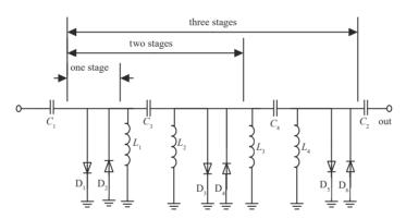
Fig.3 Main limiting circuit with different stages 图 3 不同级数主限幅电路
