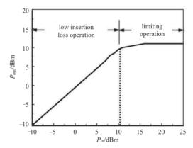
Fig. 2 Typical input and output power curve of PIN limiter 图 2 PIN 限幅器典型功率输入输出曲线
