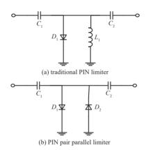
Fig.1 PIN limiter of single stage 图 1 单级 PIN 限幅器
