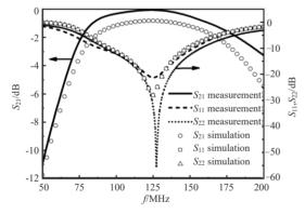
Fig.11 Comparison between simulation and measurement of S parameter 图 11 S参数仿真与测试结果对比
