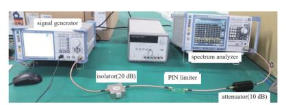
Fig.10 Measurement of limiting performance 图 10 限幅性能测试
