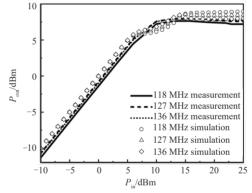
Fig. 12 Comparison between simulation and measurement of limiting performance
