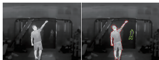
Fig.3 Infrared pose dataset annotation sample 图3 红外姿态数据集标注样例
