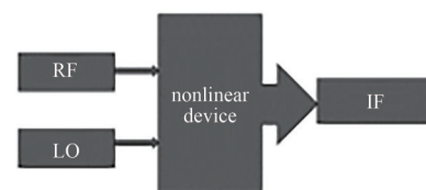
Fig.14 Working principle of mixer 图 14 混频器工作原理
