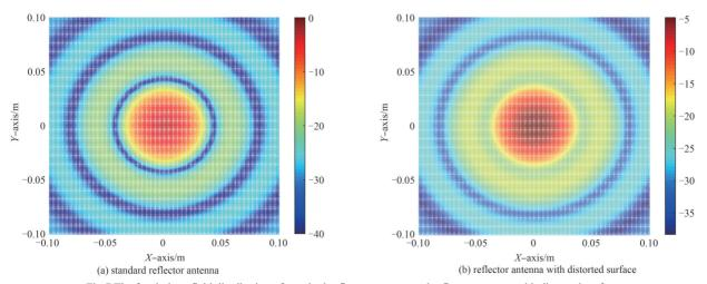
Fig.7 The focal plane field distribution of standard reflector antenna and reflector antenna with distorted surface 图 7 标准反射面天线和形变反射面天线焦面场分布
