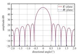
Fig.8 Performance of standard reflector antenna illuminated by Gaussian feed 图 8 高斯馈源照射标准反射面天线性能
