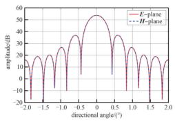
Fig.9 Performance of standard reflector antenna illuminated by phased array feed 图 9 相控阵馈源照射标准反射面天线性能
