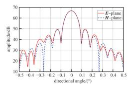
Fig.6 Performance of phased array feed with disturbance 图 6 受扰动时的相控阵馈源性能
