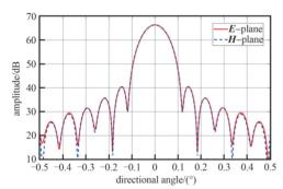
Fig.1 Performance of Gaussian feed without disturbance 图 1 无扰动时的高斯馈源性能
