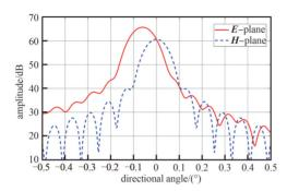
Fig.5 Performance of Gaussian feed with disturbance 图 5 受扰动时的高斯馈源性能
