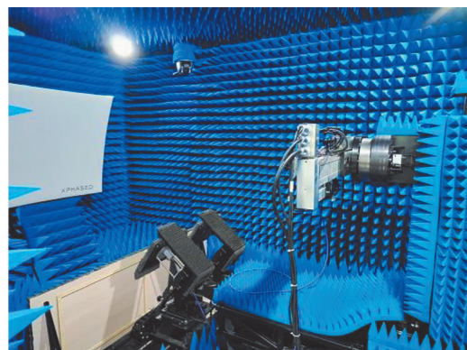
Fig.6 Schematic of compact range quiet zone test 图6 紧缩场静区性能测试示意
