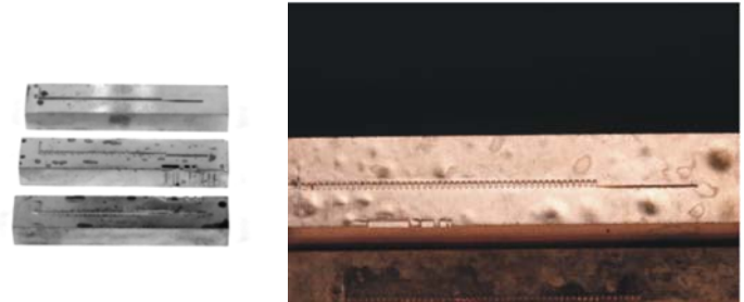
(a) before annealing in pure hydrogen (b) after annealing in pure hydrogen
