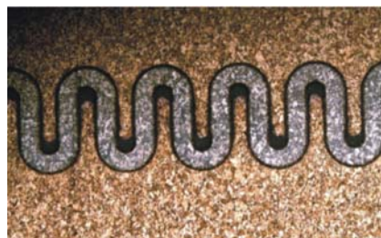
Fig.10 Image of resist molds patterned by over-exposure dose 图 10 过曝光量时形成的光刻胶模
