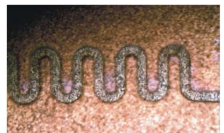
Fig.11 Image of resist molds patterned by optimal exposure dose 图 11 正常曝光时形成的光刻胶模
