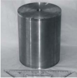
Fig.6 Picture of the permanent magnet for BWO 图 6 返波振荡器用磁系统照片
