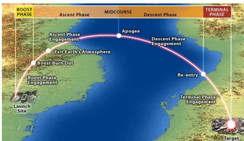
Fig.6 Schematic of ballistic target in flying course
