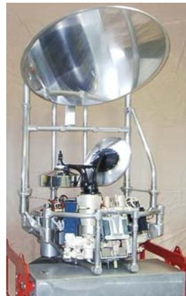
Fig.2 Russian microwave imager/sounder MTVZA-GY for spacecraft "Meteor-M",with three frequency channels around 183 GHz<sup>[10]</sup>
