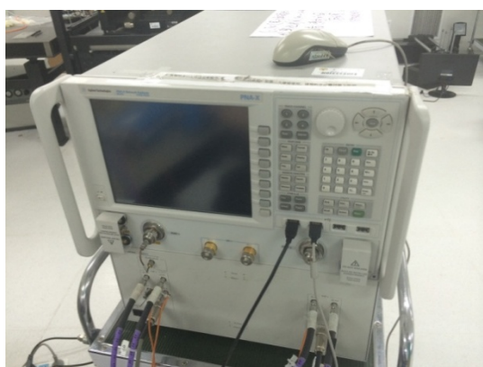
Fig.5 Agilent N5245A vector network analyzer and the frequency extended model for test
