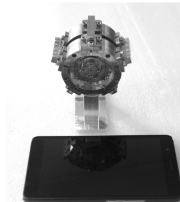
Fig.9 Photo of the 5-way coaxial-waveguide combiner 图 9 实物照片
