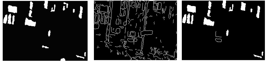
(a) region analysis of multi-scale fusion (b) edge detection of multi-scale fusion (c) extracted buildings
