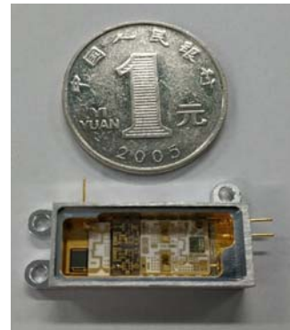
Fig.7 Picture of the Limiting and LNA 图 7 限幅低噪放外形图
