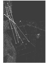
Fig.6 Non-homogeneous SAR image based on SIFT features 图6 非同源SAR图像的SIFT特征算法匹配结果
