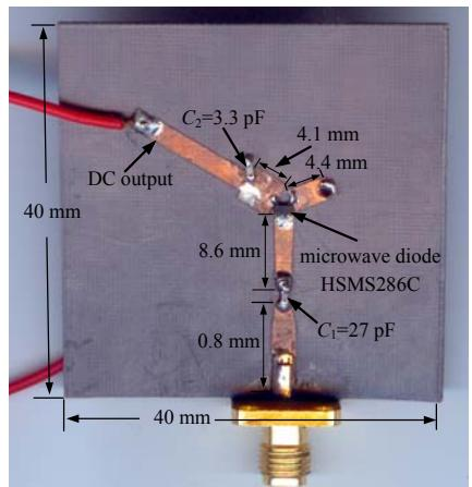
Fig.3 Microwave diode rectifier
