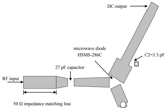
Fig.2 Optimized rectifier circuit
