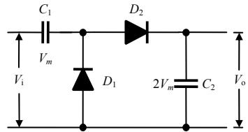
Fig.1 Diagram of voltage coupling rectifier circuit
