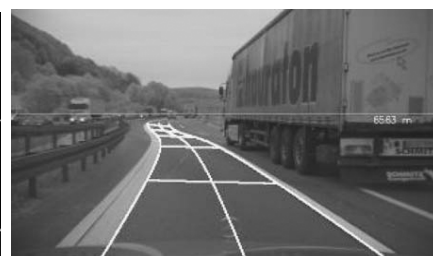
Fig.4 Lane tracking on marked highway utilizing a B-spline lane model 图4 基于B样条模型的弯曲道路检测
